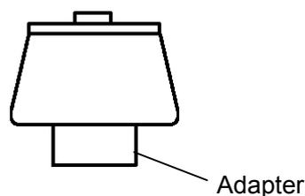
**NOTE** The rotors without the adapters are not available for this centrifuge.
