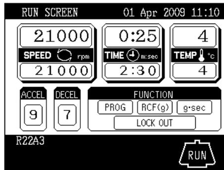
Fig. 2-2-5 Display panel of CR21GⅢ(When the lockout system has been set)
