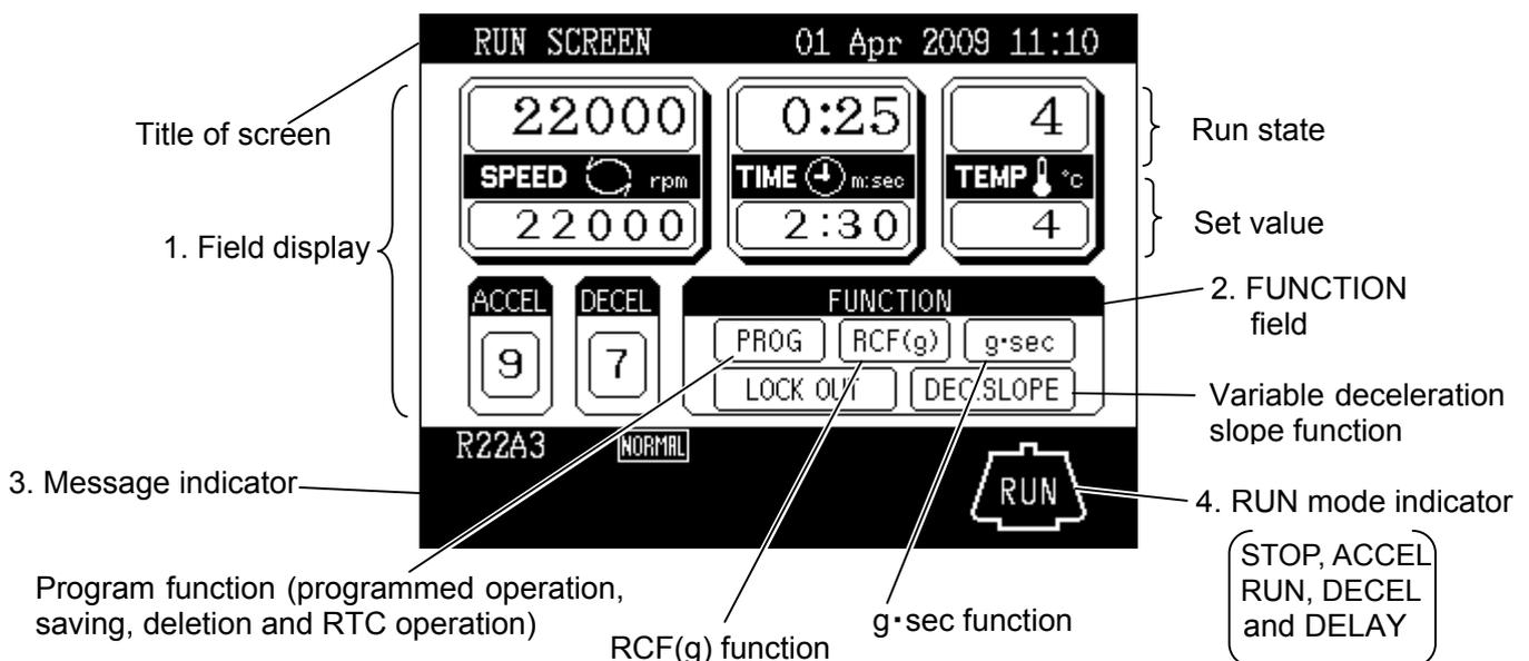
Fig.2-2-3 Display panel of CR22 GⅢ (When the lockout system has been set)
