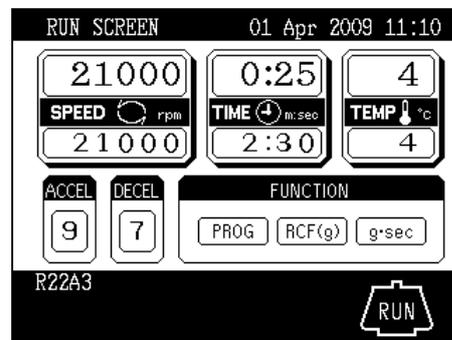
Fig. 2-2-6 Display panel of CR21GⅢ(When the lockout system has not been set)
