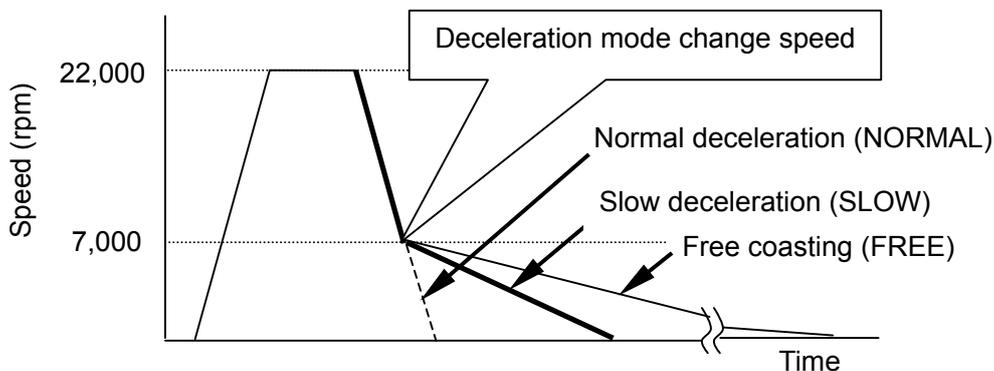
Fig. 3-3-5 Example of operation using the variable deceleration slope function
