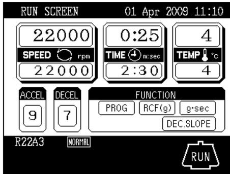
Fig. 2-2-4 Display panel of CR22GⅢ(When the lockout system has not been set)
