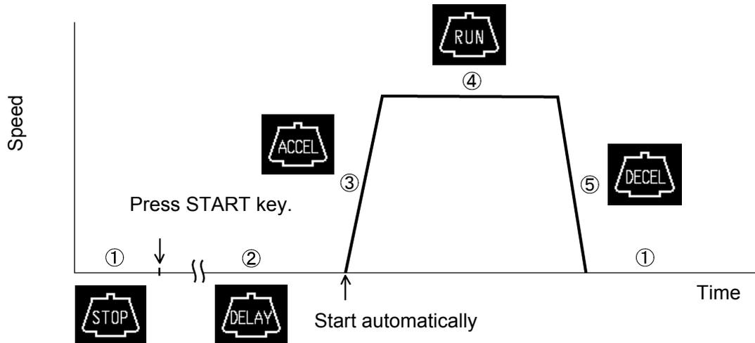
Fig. 3-3-4 Operating mode (RTC)
