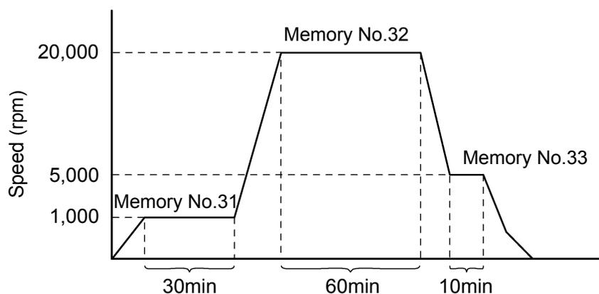
Fig. 3-3-2 Details of an example step-mode operation
