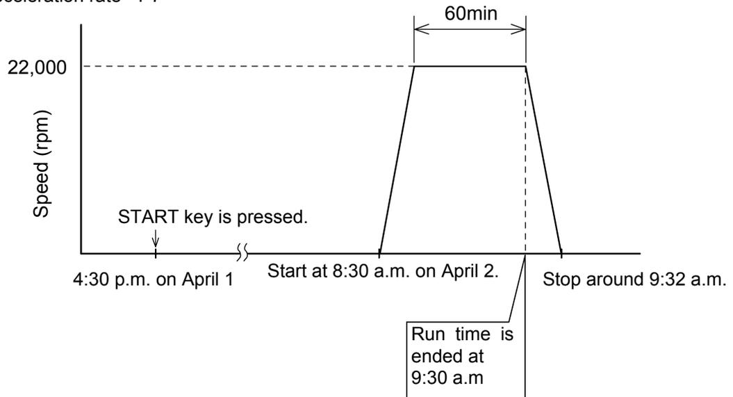
Fig. 3-3-3 Example of RTC operation
